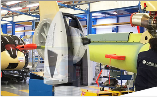
Portable CMM Laser Trackers like the Hexagon Leica Absolute Laser Tracker AT960 are popular for measurement and computer-aided assembly of large parts and assemblies such as aircraft and automotive tooling.
