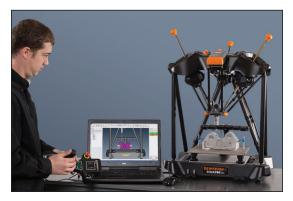
Verisurf Software works with all portable, and stationary CMMs; the part being inspected and the CMM are presented in a virtual on-screen environment with GD&T definitions in full view, providing a seamless interface between the physical part and the nominal CAD model,
