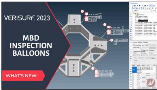
Verisurf software integrated FAIR features – Verisurf metrology software automatically creates balloon IDs and assigns them to dimensions and callouts in the 3D model.
