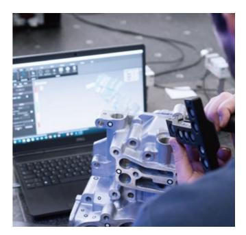
**Contact probing:** It can be paired with a portable CMM K-Probe to probe inaccessible areas and complex parts, offering comprehensive and precise 3D solutions.
