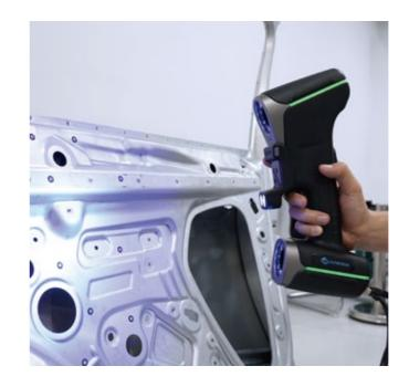
**Intelligent edge inspection:** It boasts an optional module for intelligent edge inspection. With high-precision gray value measurement, users can inspect closed features precisely and obtain repeatable measurement results.
