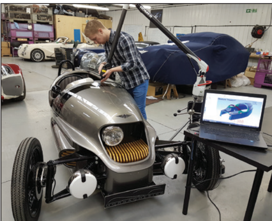
Handcrafted cockpit details of the Morgan EV3 are reverse engineered to a 3D CAD model using Verisurf Reverse Software and Romer portable CMM with laser scanner.
