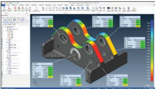
Verisurf inspection software reads in intelligent GD&T data, which can be edited, including adding additional annotations. Any deviation from nominal is presented in real-time during inspection using color mapping.
