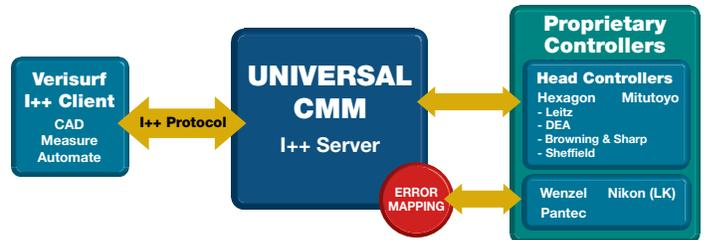
CMM—they can continue to use legacy inspection programs if needed and still enjoy the benefits of using Verisurf. Inspection programs created in Verisurf for a CMM can also be used on portable systems. Human and technology resource utilization improves substantially when all measuring devices can be operated with the same metrology software and skill sets.
