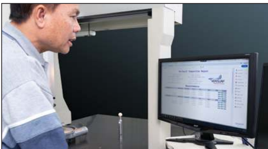
Operator completing first article inspection report using Verisurf Software.
