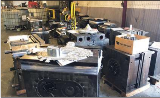
The proof is in the part; molds are designed with thermal allowances mold quality is determined by part quality. Molds are stored with a sample of the most recent part shot.
