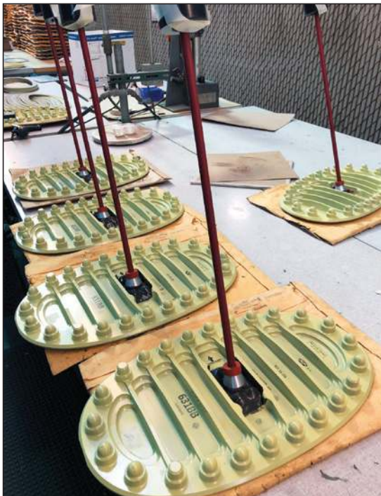
Die cast aerospace fuel cell inspection ports, assembled with float gauge component.
