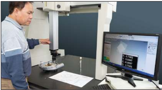
Verisurf Software works with all CAD files, including 2D CAD, 3D CAD models, and paper drawings. Shown, Verisurf Software is used to verify a finished part against a paper drawing.
