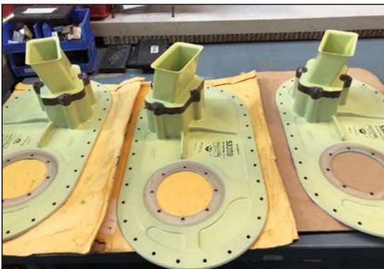
Die cast aerospace inspection ports, assembled with Die cast flame arrestor component.
