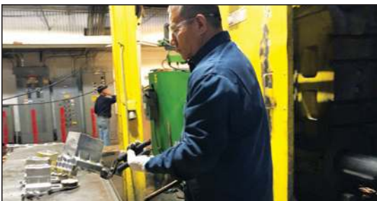
Following visual inspection of the first shot, the part is allowed to cool and stabilize before being dimensionally verified using Verisurf Software.
