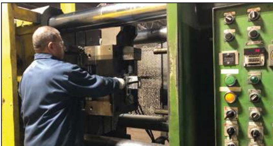
Releasing the part from the die cast mold.
