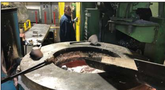
Die cast machine operator prepares for initial test shot of a new die cast mold.
