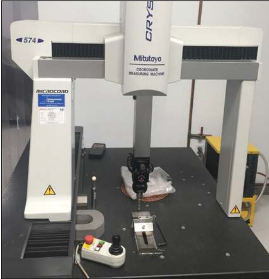
Legacy Mitutoyo CNC CMM being driven by Verisurf software.
