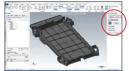
Software screen shows Verisurf Device Interface (VDI), indicating Verisurf Universal CMM I++ Interface is being used to control the legacy Wenzel CMM.
