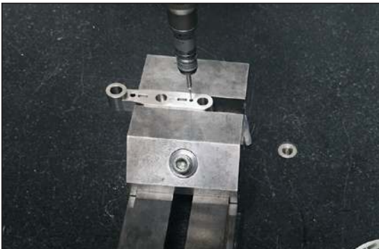
Close up of a production part being inspected by Verisurf software, running a legacy Mitutoyo CNC CMM.
