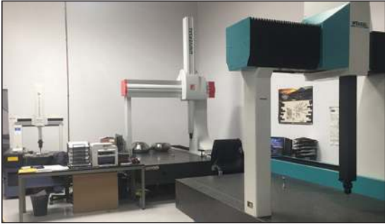
The Mitutoyo, Wenzel and Coord3 programmable CNC CMMs shown are all driven by Verisurf software which reduces training costs while improving consistency in the inspection and reporting process.
