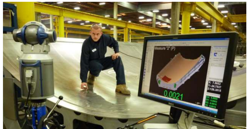
Laser projector guided profile measurement of a composite layup tool using Verisurf Project and a portable laser tracker.
